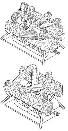
Figure 17 - Placement of Top Logs Logs (Number and style may vary)
